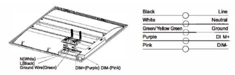
3. Please refer to the following wiring diagram when connecting the emergency driver.
