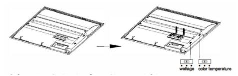
2. Connect coordinating wires. Secure driver covers to fixture.
