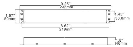
This emergency driver is designed for a product with internal driver. This emergency driver have been evaluated to and found compliant to UL 924. The emergency pack assembly is accepted as a component of a luminaire where the suitability of the combination shall be determined by UL or Authorities Having Jurisdiction. The as installed performance of the system must meet or exceed all Federal State, and Local code requirements.
