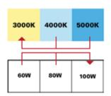
\*Remove glass cover to select desired color temperature and wattage.
