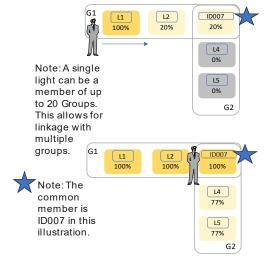
Note: For a light to respond to the 'Link' command from other lights in the same group, the 'Motion Sensor' function must be enabled for this light, even if the light does not have a motion sensor connected to it.
