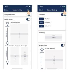
The sensor settings can be changed as a Group by selecting the lower right hand motion symbol.
