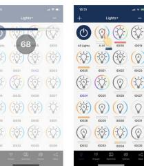
3. Lightly slide a finger up or down over a light's icon to adjust the color temperature.
