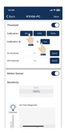
1. For photocell sensors, the default ON/OFF threshold is 10/60 fc. User may change the thresholds. Click the button of 5fc/50fc/100fc will set 5/50/100 fc as ON threshold respectively and the lights will turn on/off several times to auto-calculate the OFF threshold. User may input a specified fc value as ON threshold and select the "Cal" button to calculate the OFF threshold based on it.
