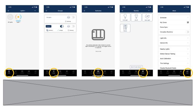
"Lights" shows all lights that are connected to the app. It allows the user to view and control individual lights. "Groups" allows user to create and manage groups.
