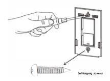
Step 6: Attach the wall plate.
